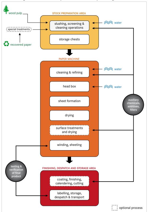
Figure 2 – Schematic Representation of the Papermaking Process
